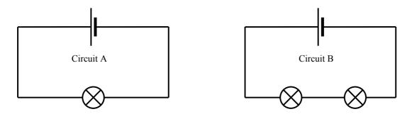
In circuit A the brightness of the bulb is normal.
