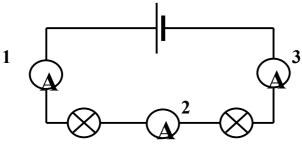
In this circuit the ammeter at position 1 reads 0.3 Amps.
